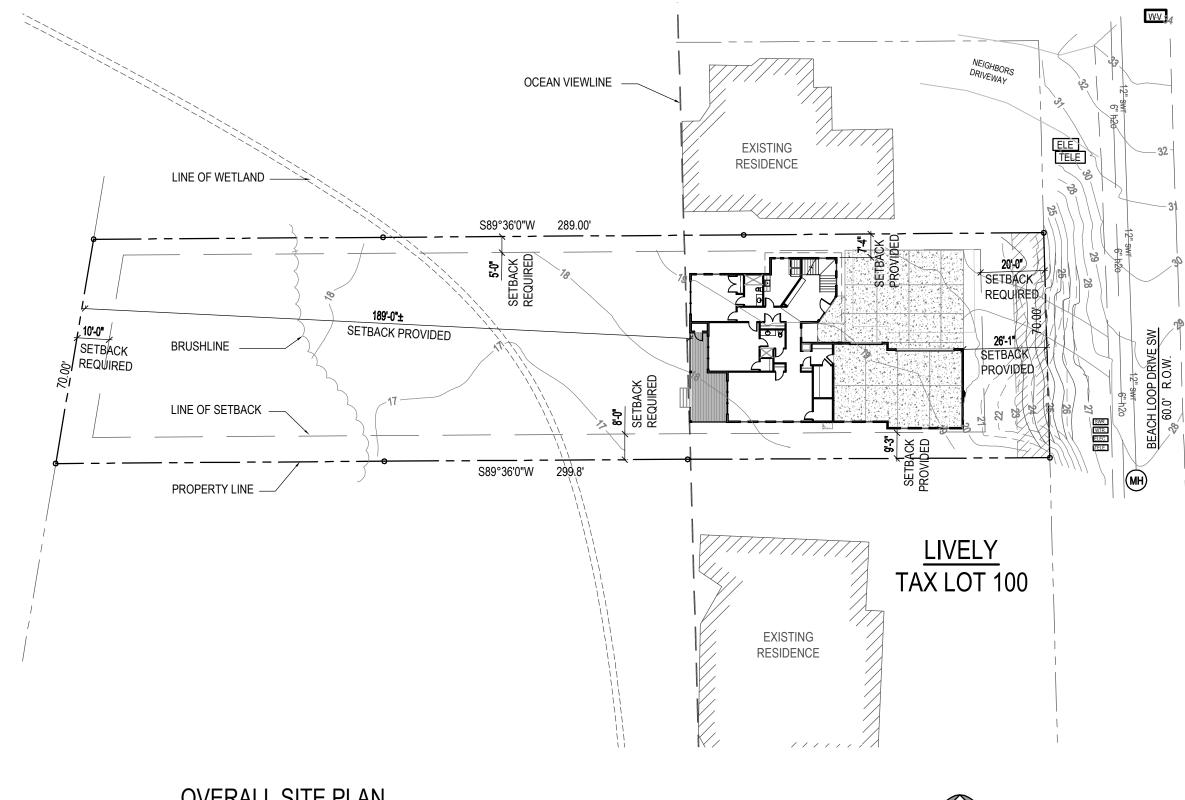
FLOODPLAIN DATA FIRST FLOOR ELEVATION 22.0' BASE FLOOD ELEVATION 21.0' AVERAGE NATIVE GRADE 19.5' WEST 20', 19' 19' 18' NORTH 20', 20', 20', 20' EAST 20', 20, 20', 20' SOUTH 20', 18', 19'
